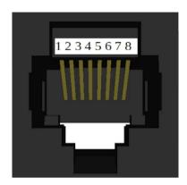
Pinout of serial connector S1,S2 on the back side.
