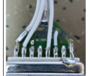
From left to right: Pin 8: Batterie plus Pin 7: Speaker + Pin 6: Mikrofon R Pin 5: Ext. NF Pin 4: Speaker minus (not GND) Pin 3: Mikrofon L Pin 2: TX Remote
