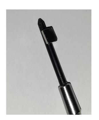
remove the 4 Corner M3 sunken head screws. again use a magnatized screw driver, a small magnet near the tip of the philipshead like in the picture is also okay.
