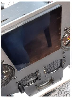
press the LCD inside make sure the 3 pulltruding rectangular strip align with the holes
