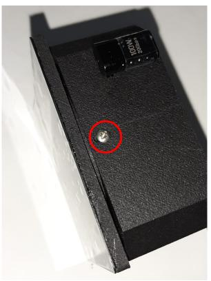
Remove the 3 M2.5 screws from the sides use a magnatized philipshead screwdriver
