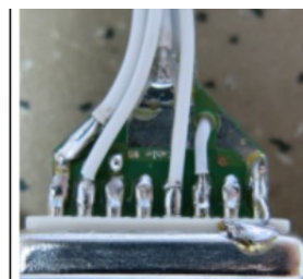
From left to right: Pin 8: Batterie plus Pin 7: Speaker + Pin 6: Mikrofon R Pin 5: Ext. NF Pin 4: Speaker minus (not GND) Pin 3: Mikrofon L Pin 2: TX Remote
