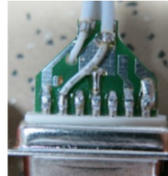
From left to right: Pin 9: GND Mikrofon Pin 10: PTT-L Pin 11: PTT-R Pin 12: Intercom with Bridge to Gnd Pin 13: RX Pin 14: Headset Pin 15: connected with Pin 8 Batterie+
